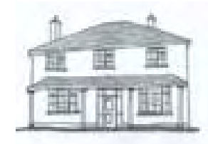
Classical 'mock' hipped portico
